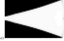
$f=171.96 \text{ kip ft} (233.15 \text{ kN} \cdot m)$   $f=1478.44 \text{ kip ft} (2004.49 \text{ kN} \cdot m)$   $f=81155.77 \text{ kip ft} (110032.40 \text{ kN} \cdot m)$ Figure 8. Optimized design for the cantilever beam example for fixed angle  $\theta=90^{\circ}$ ,  $\beta=1$ , and decreasing Young's modulus by a factor of (a)  $\alpha=0.1$ , (b)  $\alpha=10^{-2}$ , and (c)  $\alpha=5\cdot10^{-5}$ .
