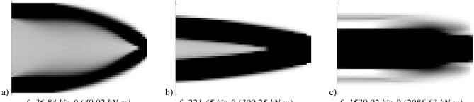
f=36.84 kip ft (49.92 kN·m) f=221.45 kip ft (300.25 kN·m) f=1539.02 kip ft (2086.63 kN·m)Figure 7. Optimized design for the cantilever beam example for fixed angle  $\theta=0^\circ$ ,  $\beta=1$ , and decreasing Young's modulus by a factor of (a)  $\alpha=0.1$ , (b)  $\alpha=10^{-3}$ , and (c)  $\alpha=10^{-6}$ .
